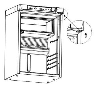
4.Remove the hinge shaft on the right side and install it on the left side, requiring it to be installed in place.
