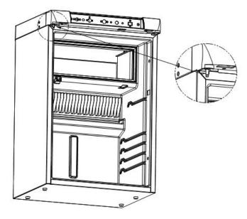
5. After the door body is installed in place, install the removed lower hinge on it.
