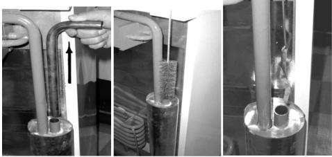
Examine the soot flue on the refrigerator. Be sure there is no soot and keep the flue clean. If there is heavy soot in the flue, the burning efficiency would be impaired. Thus, with the special brush supplied, you should clean the soot regularly (refer to the picture)
